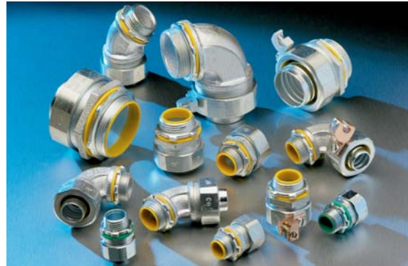
Liquidtight fittings come in a wide range of sizes in straight, 45° and 90° styles. They are available in steel, aluminum, zinc die cast or non-metallic with or without insulated throats and aluminum or copper grounding lugs.
