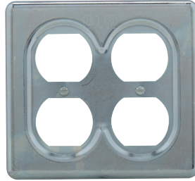
For duplex convenience receptacles, standard and 2-wire, 3-pole grounding; hole diameter 1 11/32 "
