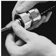
3. Mix sealing compound and pack conductors over armor.
